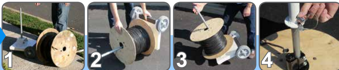
Feed the spool rod through the reel's ID and use the spool rod as a mechanical advantage for lifting the cable reel in upright position.
